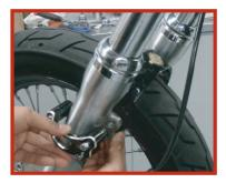
4. Install the supplied washers (3) and nylock nuts (4) and torque to 17 ft-lbs.
