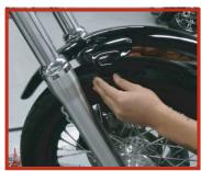
3. With the fender removed clean and inspect the mating surfaces and install the RSD Tracker fork brace (6) using the supplied inner spacers (9), outer clamps (7), front spacers (8), and bolts (2).
