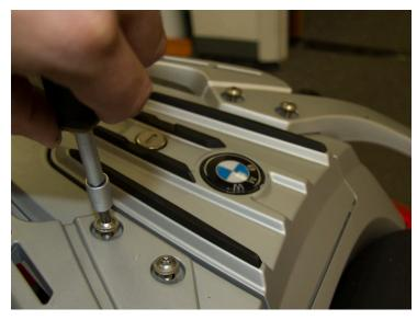
Using your T30 driver, remove the (4) T30 screws and set aside. You will not be reinstalling these screws.
