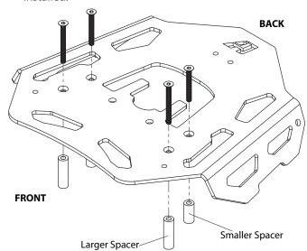
Install luggage rack, spacers and screws. Start with the rear spacers and screws (smaller screws and spacers) and finish with the front spacers and screws. Tighten all (4) screws completely with M4 allen driver.
