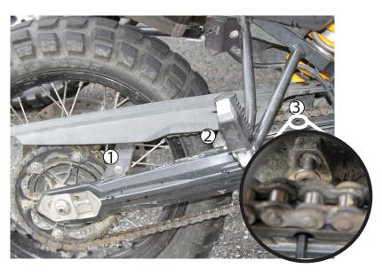
2 Install the AltRider guard with the (2) OEM screws. Torque to 10 nm or torque.
