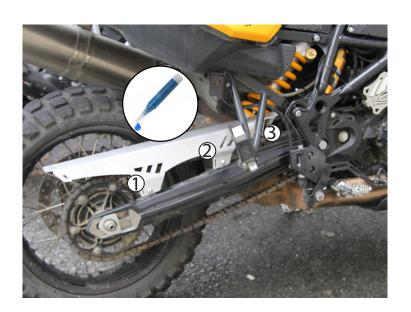
Install the (2) AltRider provided M6 x 25 mm screws to positions 1 and 2 using an M4 allen driver also add a drop of thread locker to each. Tighten all (3) screws to 10nm of torque.
