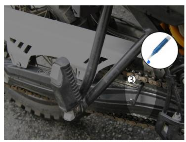
Install the new AltRider chain guard and begin tightening the forward most M6 screw using the T27 torx key. Add a drop of thread locker and then make this screw snug but do not torque down just yet.
