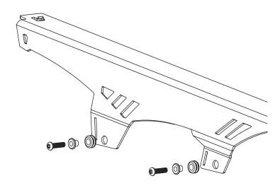
Install the (2) AltRider provided rubber grommets and (2) custom shoulder washers into the AltRider aluminum chain guard as shown. Sometimes it is easier to install the rubber grommets when you have the lubricated.
