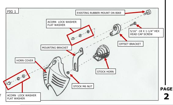
Remove the M6 nut that secures the horn to the stock mount and cover. Set this nut aside, it will be reused. Remove the horn from the stock cover. Adjust the position of the offset mount to approximately 5 o'clock (this will center
