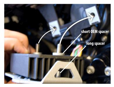
We recommend holding the assembly together as shown then, using a 4mm allen tool, tighten the (2) M6s. Tighten firmly, do not crank on these!
