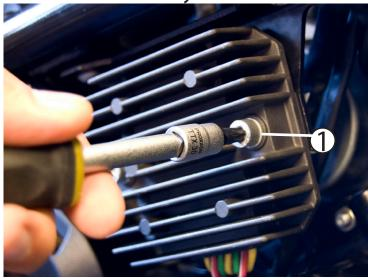
Using a T30 torx tool, remove the (2) fasteners that hold the voltage regulator in place.
