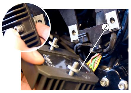
Remove the voltage regulator, be careful not to lose track of the two spacers shown above. You'll be reusing those in a second.
