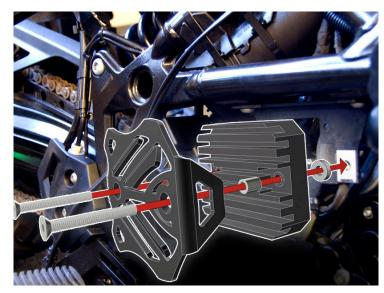
3 Use the exploded view above as a guide for assembly. The two OEM spacers are important, so place them as shown above!
