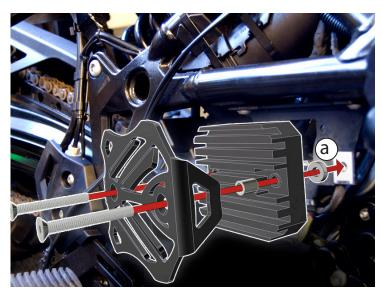
Use the exploded view above as a guide for assembly. Exploded view is of F800 but TR650 install order is identical with the exception of the oem spacers (a), these are not used. Using a 4mm allen tool, tighten the (2) M6s.
