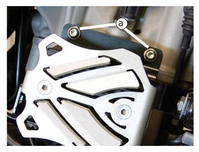
Install the (2) M5 x 12 Torx screws with (2) M5 washers into now empty holes on OEM bracket using a T25 driver (a). Tighten all the way.
