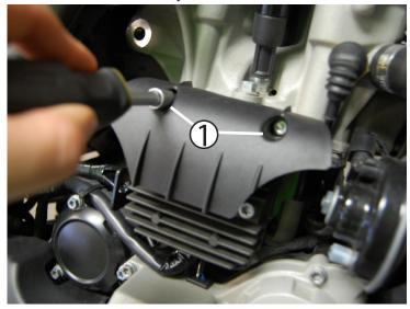
Using a T25 torx tool, remove the (2) fasteners that hold the OEM voltage regulator guard in place. You no longer need these fastners.
