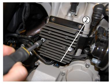
Using a T30 torx tool, remove the (2) fastners holding the voltage regulator in place. You no longer need these fastners.
