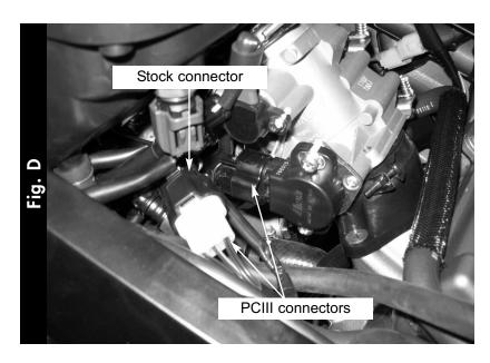
Plug the PCIII connectors in-line of the stock wiring harness and TPS (Fig. D).
