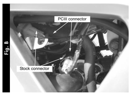
5 Unplug this connector and plug the Power Commander connectors in-line (Fig. B).
