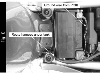
9 Attach the ground wire from the Power Commander to the negative side of the battery (Fig. E).
