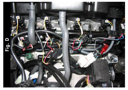
Plug the PCIII wiring harness in-line of the stock harness and injectors (Fig. D).
