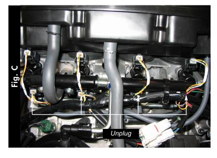
6 Unplug the stock wiring harness from the lower injectors (Fig. C).
