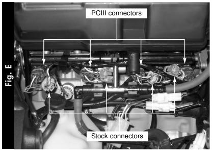
5. Plug the PCIII connectors in-line of the stock injectors and wiring harness.
