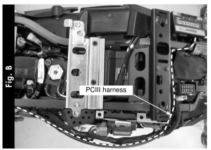
3 Lay the PCIII in the tail section and route the harness along side the stock wiring harness towards the throttle bodies (Fig. B&C).
