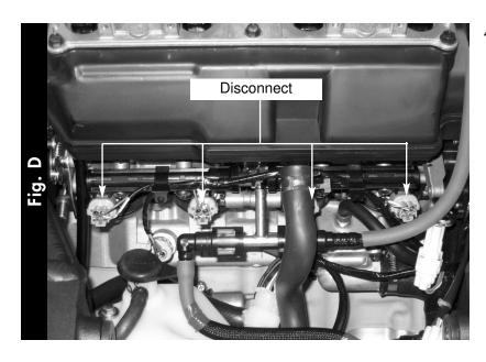
4. Disconnect the stock wiring harness from the LOWER injectors at the throttle bodies (Fig. D).
