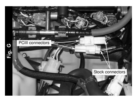
7. Plug the PCIII harness in-line of the stock wiring harness (Fig. G).
