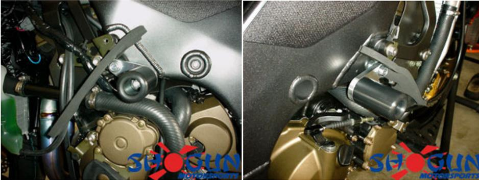
5. Install the flat offset with the 10 X 1.25 X 80 bolt; lightly tighten up bolt so you can locate the bracket so the slider puck will clear the body. (If you torque down the bolt to the OEM spec. prematurely the bracket will be too tight to move in case you need to readjust location to clear the body.)
