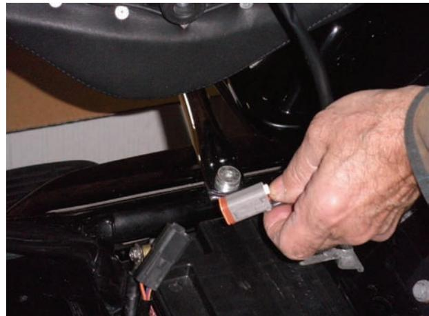
**Step 6** Check to make sure there are no folds or kinks in the wire leading from seat to receptacle before finalizing installation of seat. Engage front mounting tab first, push seat all the way forward, and insert and tighten the rear fender screw.
