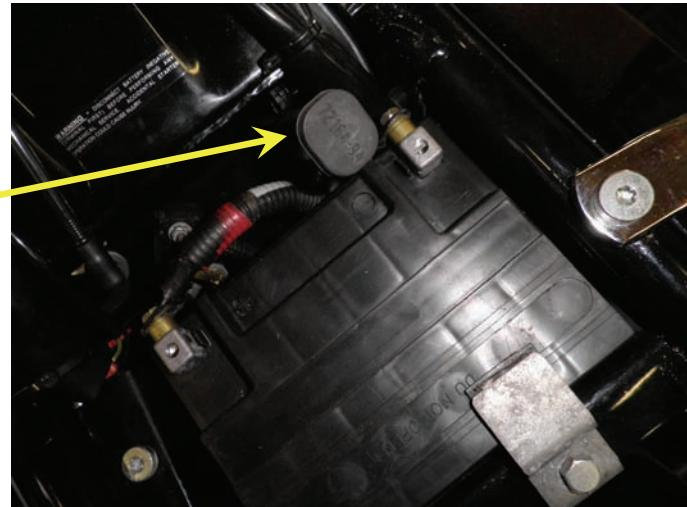
**Step 3** Remove the rubber cap from the accessory receptacle. Make sure that the receptacle is clean and free of any dirt or debris. If dirty, be sure to clean it before attaching heating plug from Mustang seat.
