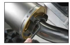
Slide the muffler assembly into the stock muffler gasket and clamp. Do not tighten this clamp until final step.
