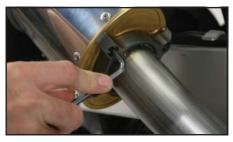
7. Securely tighten the muffler canister clamp.
