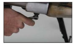
Install OEM rubber bumper to center stand bracket by twisting and pushing.
