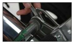
8. Securely tighten the muffler joint clamp to the stock collector.
